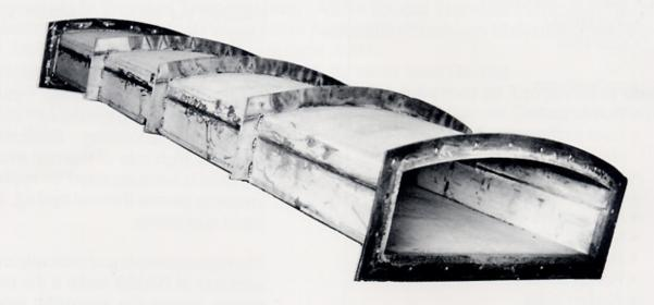
Muffle of 3/16" (4.76mm) RA309 plate. Gas fired 1200-1600°F(650-870°C), endothermic atmosphere, bright annealing copper, brass and steel. Typical life 4-5 yrs.
